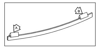
3. Hold the wiper blade refill with the curved side facing downward.
